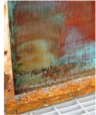
Corrosion Effects on a typical Copper-Copper Coil
